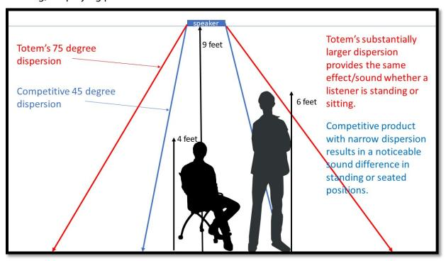
The following chart for speaker spacing was calculated using the following formula: ANGLE(dispersion) x .018 x DISTANCE (ceiling height) = SOUND COVERAGE radius
