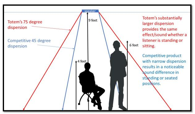
The following chart for in-ceiling speaker spacing was calculated using the following formula: ANGLE (dispersion) x .018 x DISTANCE (ceiling height) = SOUND COVERAGE radius
