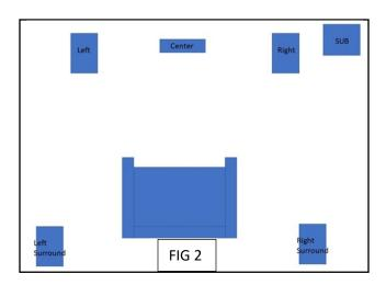
One method of finding your preferred location starts with placing the connected sub in the main listening location. Then, while content with good bass output is playing, slowly walk the perimeter of the room. You will find that bass is stronger and tighter in some locations and substantially weaker and less defined in others. When you have found the area where you feel bass sounds best, place the subwoofer there. You will now find the performance you want form the listening position.
